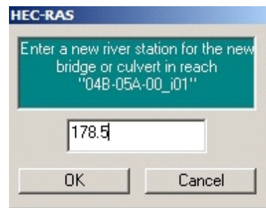
Culvert River Station Entry
